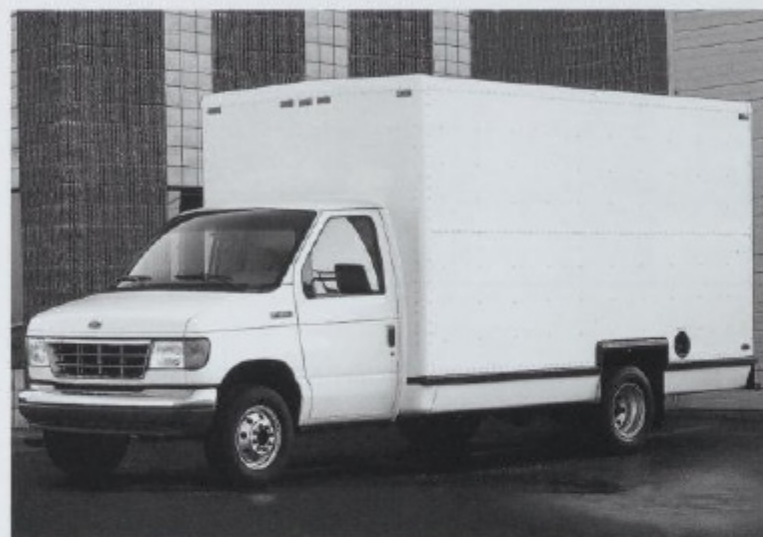
▲ The Econoline E-350 Commercial Cutaway with dual rear wheels. Payload capacities go up to 5,865 lbs. (10,700-lb. GVWR).
