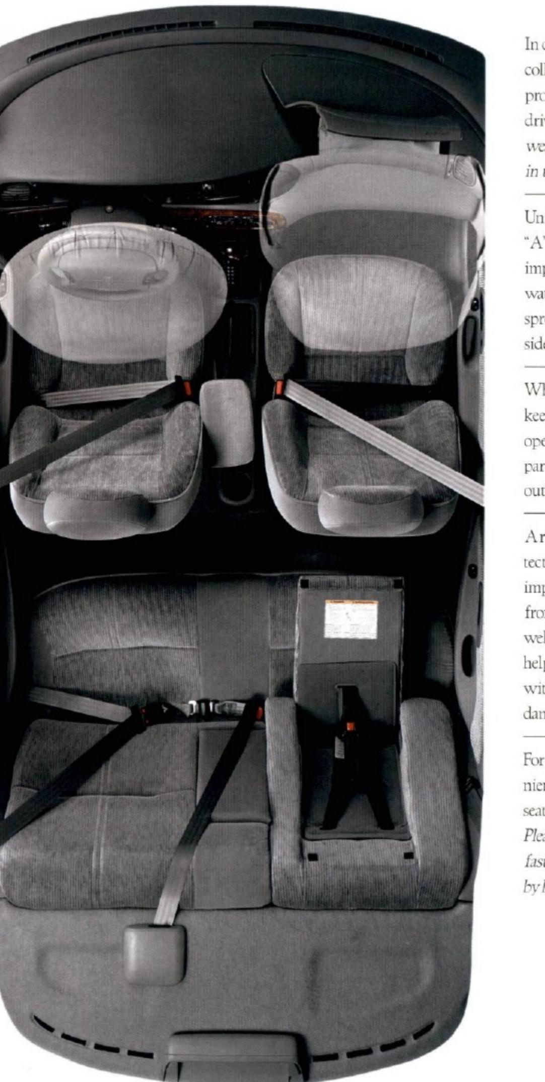
In certain moderate-to-severe frontal collisions, both air bags will deploy, providing added protection to the driver and front passenger. *(Always wear your safety belt and seat children in the rear seat.)*
