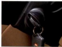
The SecuriLock™ Passive Anti-Theft System cleverly "interrogates" the ignition key, preventing the engine from being started by potential thieves.
