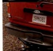
**Class III Trailer Hitch.** Designed for gross trailer load capacity of 5000 lbs., tongue weight rated at 500 lbs.
