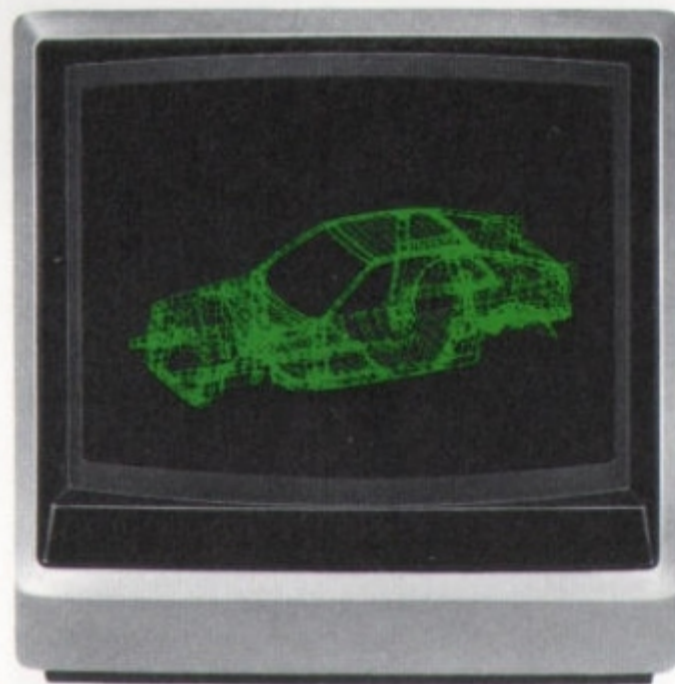
Honda's computer-aided design allows structural analysis prior to manufacture. It helps produce a strong unibody and subframe.
