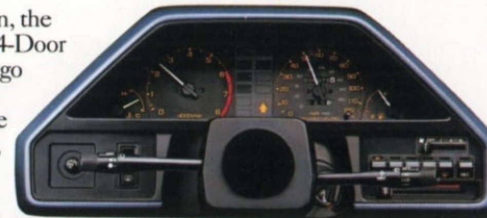
The CRX uses a tachometer and an Economy Driving Indicator (a centrally located yellow arrow), which lights to tell you when to upshift for maximum fuel economy. Like all Civics, the CRX instrumentation is laid out for easy reading.
