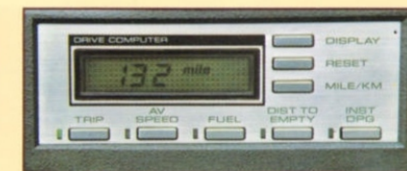
Optional Electronics Package on the Maxima GL Sedan includes a drive computer which assists you on trips and monitors trip-related functions, such as average speed and distance to empty.
