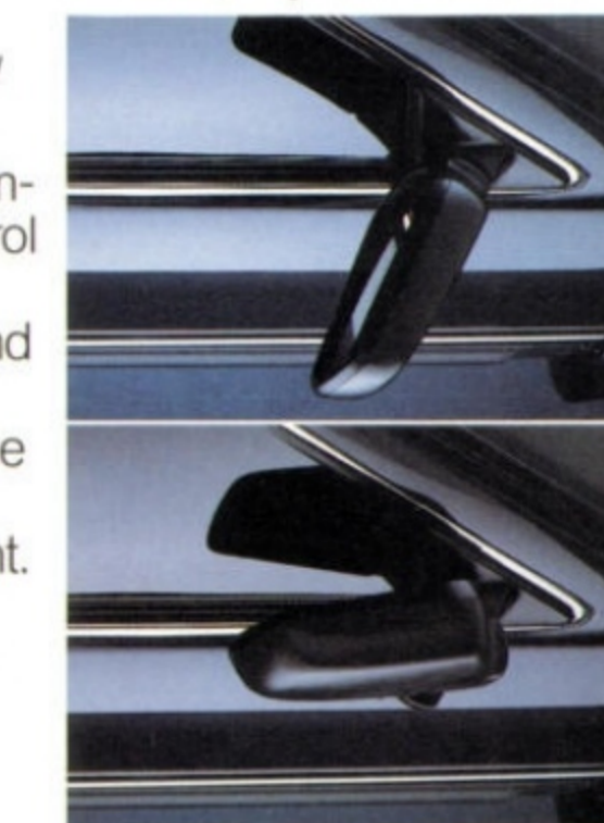
Aerodynamic mirrors are electronically adjustable and are spring loaded to fold inward.
