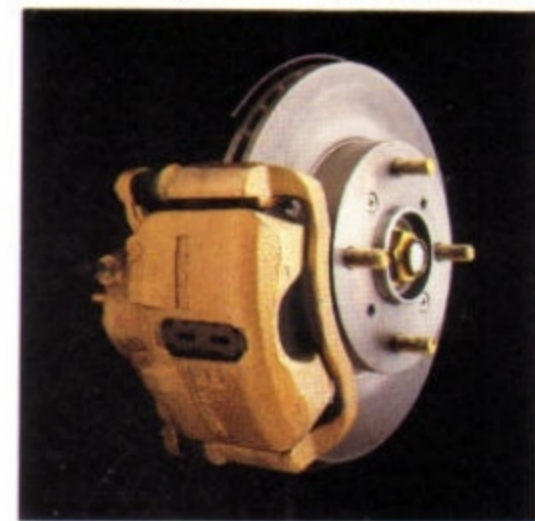
Front disc brakes are ventilated to dissipate heat.
