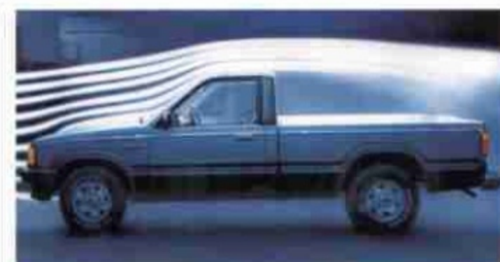
...of the new B2000 body design to reduce turbulence and wind noise and enhance fuel economy.
