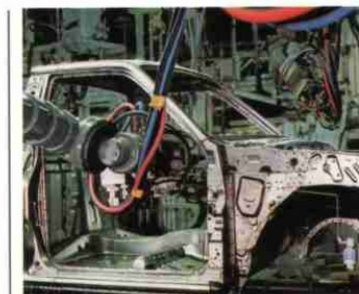
Sophisticated, computerized robots perform an intricate program of spot welds of flawless quality and precision.
