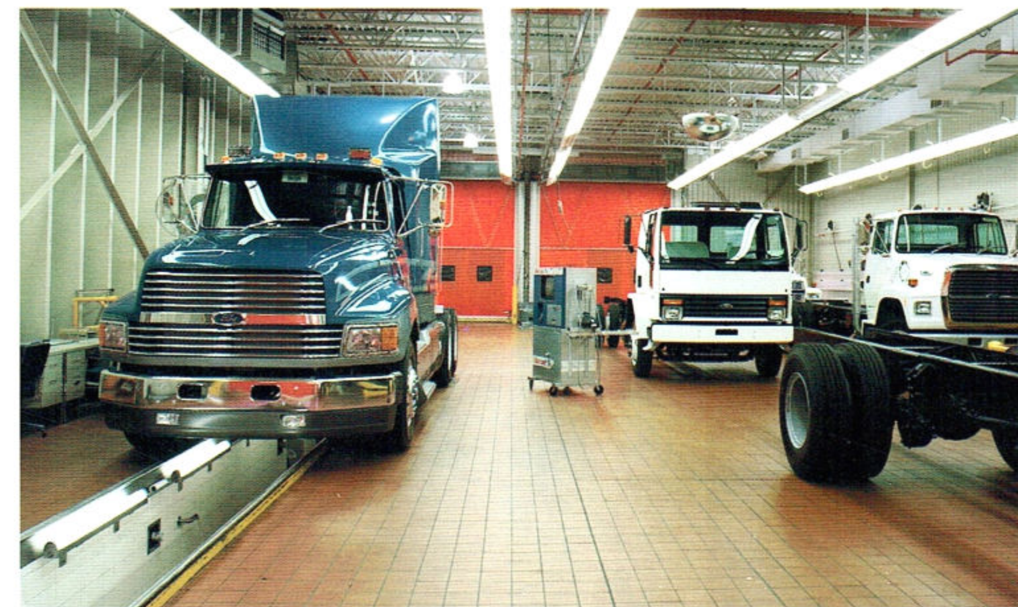
In the Audit Facility random vehicles undergo uniform product assessment. Here an AeroMax 120 is undergoing laser beam rear axle inspection.
