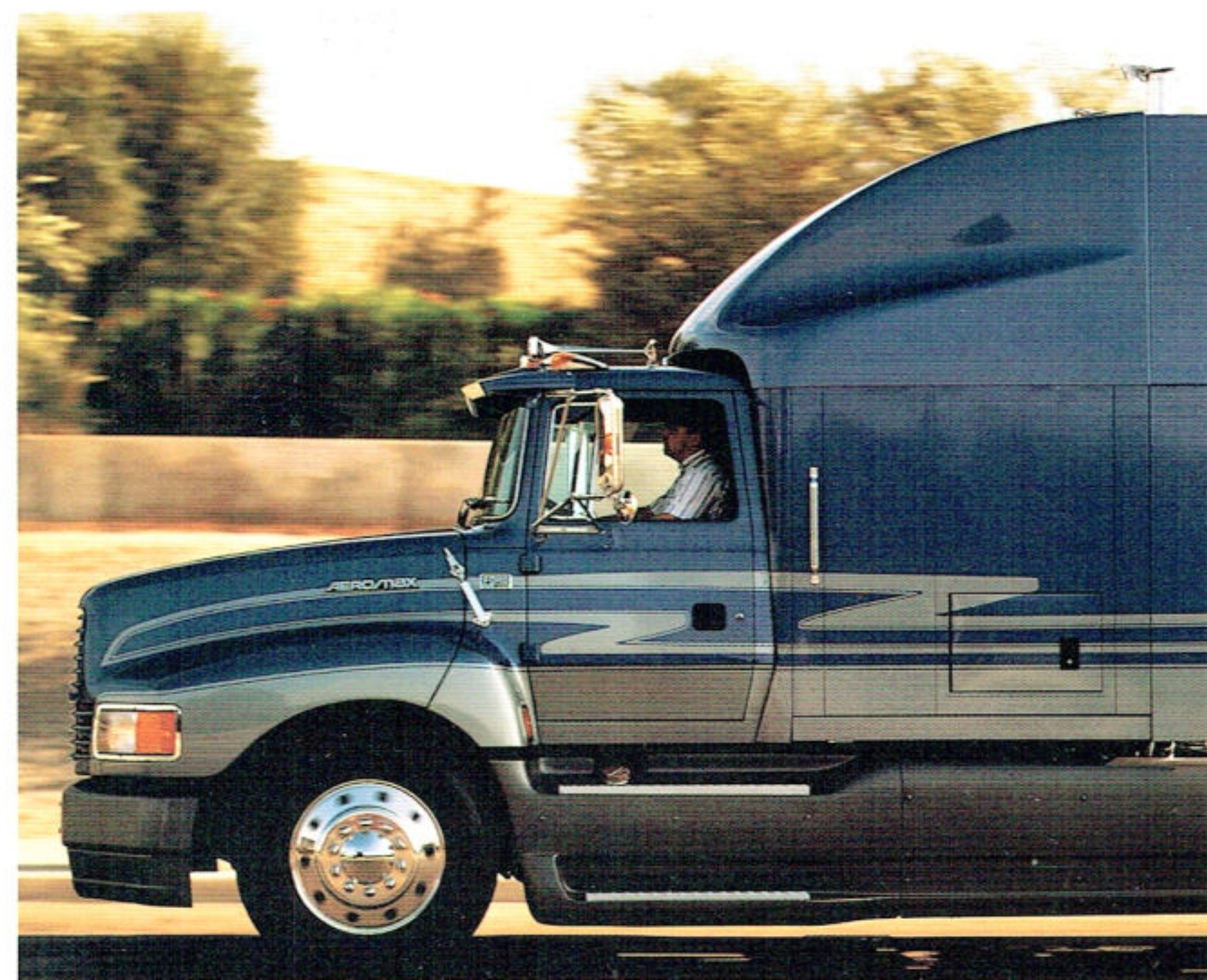
The AeroMax 120 features a set-back front axle, long parabolic taper leaf front springs plus a hydro-mount cab for impressive handling and ride.
