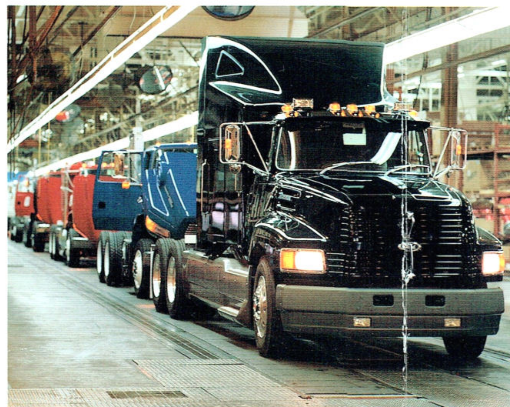
The AeroMax 120 features a set-back front axle, long parabolic taper leaf front springs plus a hydro-mount cab for impressive handling and ride.
