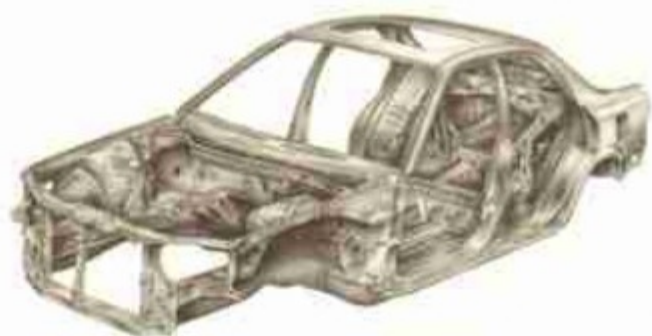
The rigid structure, with its steel-reinforced beams, contributes to impact safety. Front and rear crumple zones direct impact energy away from the passenger cabin.
