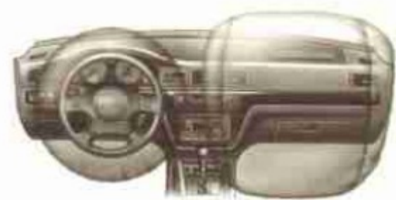
A dual air bag Supplemental Restraint System (SRS) is standard in all Acura automobiles. This system features gold-plated electrical connectors for enhanced reliability.
