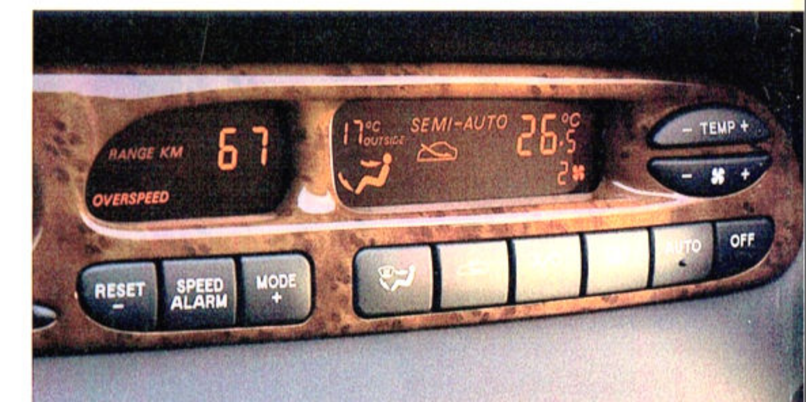
Message display centre, with trip computer, audible overspeed warning, automatic climate control and ambient temperature read-out.
