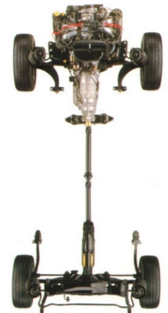
Powertrain components are laid out in a straight line and close to the chassis' centerline, giving agility while providing greater stability.
