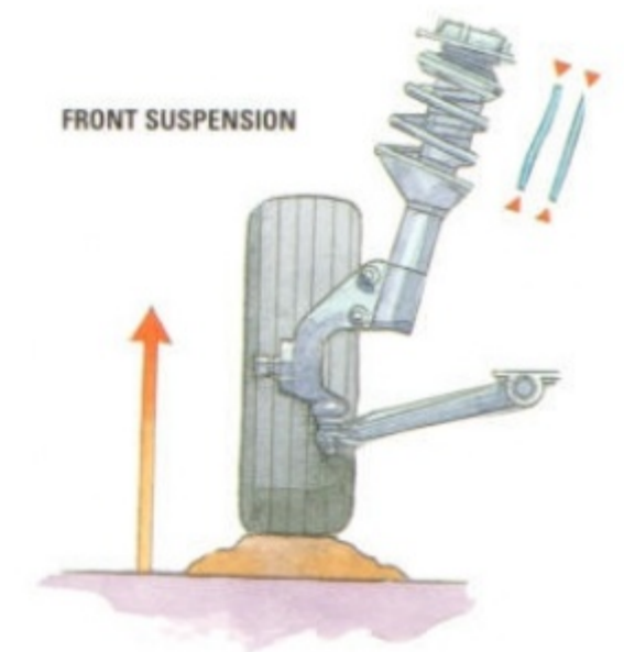
The independent suspension's long-travel, low-friction design helps absorb ruts and bumps rather than transferring them into the cabin.
