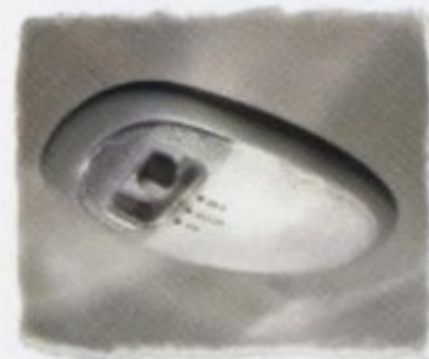
Theatre Lighting Interior courtesy lights gradually dim when doors are closed, instead of turning off abruptly.
