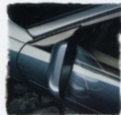
Breakaway Outside Rearview Mirrors These mirrors (standard on both Sedan and LS Sedan) are designed to allow realignment when bumped.
